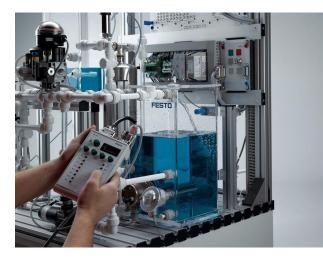
A set of educational and laboratory equipment is designed for studying continuous processes, present, for example, in oil and gas industry and food production.
